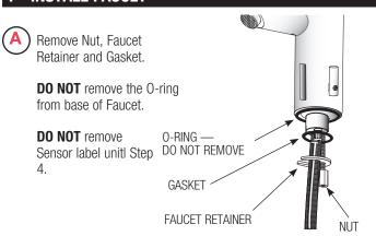
Install Faucet with O-ring into the center hole in deck or lavatory — 1-3/16" (30 mm) min. hole required.
