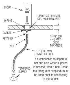
MODELS EAF-200/225\*/250/275 0.5 gpm (1.9 Lpm) Max. Flow Faucets with Hot and Cold Water Supply
