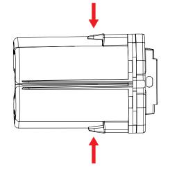
D Remove all four (4) AA-cell batteries from battery pack.
