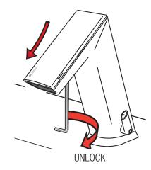
Place new crown on faucet by sliding onto spout and tightening hex screw on underside of spout.
