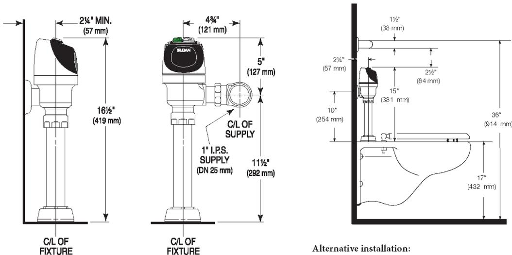
**When installing the Flushometer in an ADA compliant stall:**
