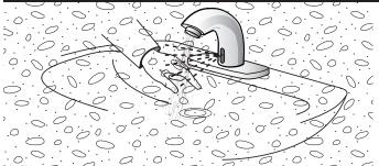
Place hands under faucet. Solenoid value should "click," LED in sensor window should blink once and water should flow from the spout.
