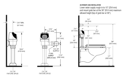
WHEN INSTALLING IN A HANDICAP STALL: Per the ADA Guildlines (section 604.9.4) it is recommended that the grab bars be split or shifted to the wide side of the stall. If grab bars must be present over the valve, use the alternate ADA installation as shown to the right.
