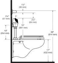
WHEN INSTALLING IN A HANDICAP STALL: Per the ADA Guildlines (section 604.9.4) it is recommended that the grab bars be split or shifted to the wide side of the stall. If grab bars must be present over the valve, use the alternate ADA installation as shown to the right.
