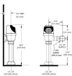
If grab bars must be present over the valve, use the alternate ADA installation as shown
