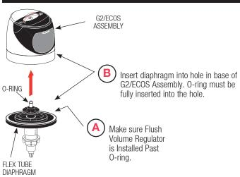
To facilitate installation, wet the diaphragm assembly (on top or completely).
