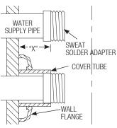
Thread Control Stop onto pipe.
