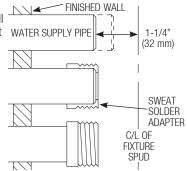
B Slide Threaded Adapter fully onto pipe.
