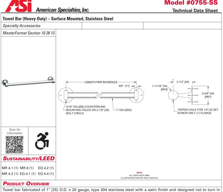
Towel bar fabricated of 1" [25] O.D. x 20 gauge, type 304 stainless steel with a satin finish and designed not to turn in support posts. Support posts fabricated of heavy solid cast brass plated to have stainless steel satin finish to match stainless steel. Variable lengths available: 0755-SS-18 – 18" [457] Length 0755-SS-24 – 24" [610] Length 0755-SS-30 – 30" [762] Length
