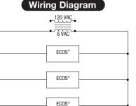
NOTE: One (1) EL-386 Transformer serves one (1) Optima Closet/Urinal Flushometer. One (1) EL-451 Transformer serves up to six (6) Optima Closet/Urinal Flushometers. 18 gauge wire (not supplied) required from transformer to flushometers.
