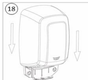
18 Mount the dryer over the Plug-in base with a from top to down movement
