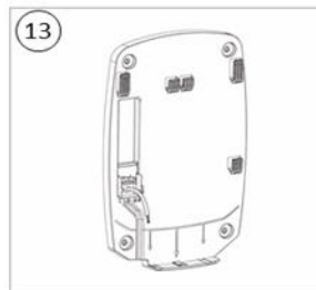
13 Route the wires through the Plug-in base as shown on the picture
