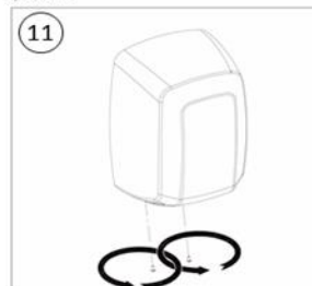
11 Screw the cover fixing screws (x2) Your dryer is now ready to be used on a Plug-in base
