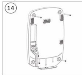
14 Screw the Plug-in base to the wall (x4)
