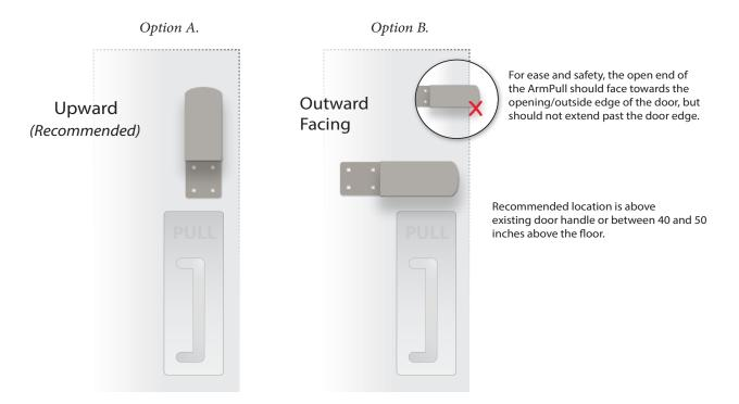
Place the ArmPull above the existing handle in desired orientation and location. Clamp or hold it to the door. If using option B., be sure that no part of the ArmPull is projecting past the edge of the door.
