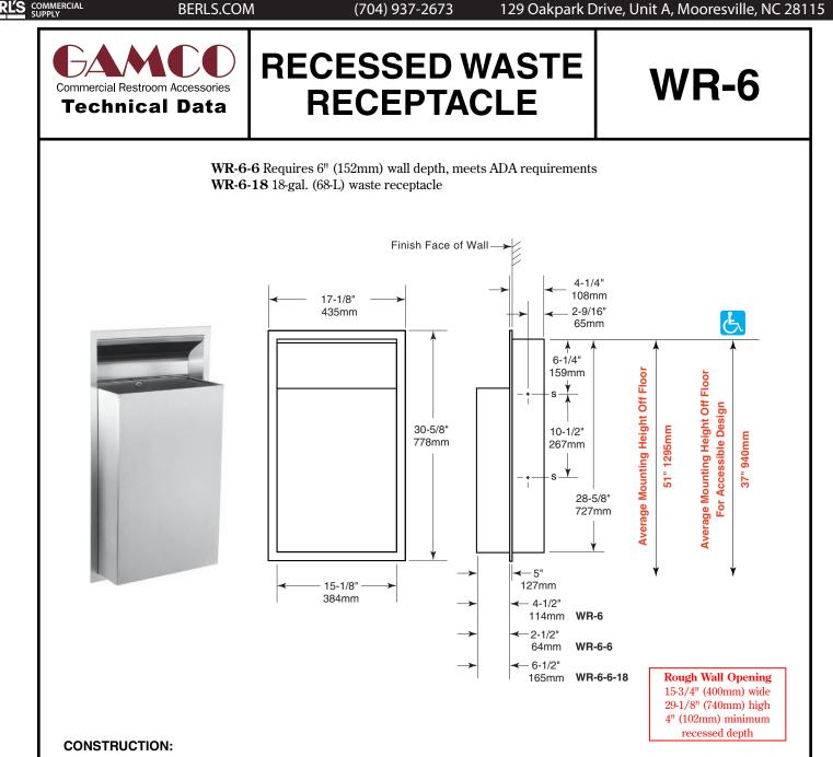
Cabinet — Fabricated of type 304 stainless steel with exposed surfaces having a #4 satin-finish.
