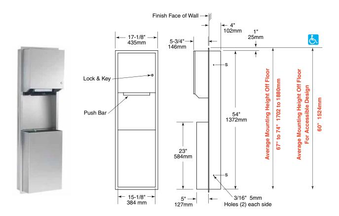
Rough Wall Opening 15-3/4" (400mm) Wide 54-3/4" (1391mm) High 4" (102mm) minimum recessed depth
