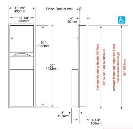
Rough Wall Opening 15-3/4" (400mm) wide 54-3/4" (1390mm) high 4" (102mm) minimum recessed depth
