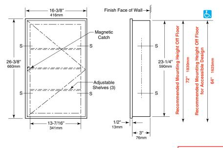
Rough Wall Opening 14" (355mm) wide 23-5/8" (600mm) high 3-1/2" (89mm) minimum recessed depth
