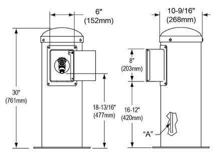
A = 1/2" O.D. UNPLATED COPPER TUBE CONNECT SHUT OFF VALVE BY OTHERS
