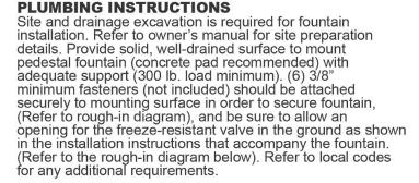
Locate and install plumbing through ground as required. Assemble fountain to prepared site and mounting pad.
