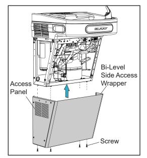
**Note:** While the side access wrapper is being secured, verify the upper profile (left, front, and right side) of the wrapper frame slides up and under the plastic basin shroud assembly for a tight fit (as shown).
