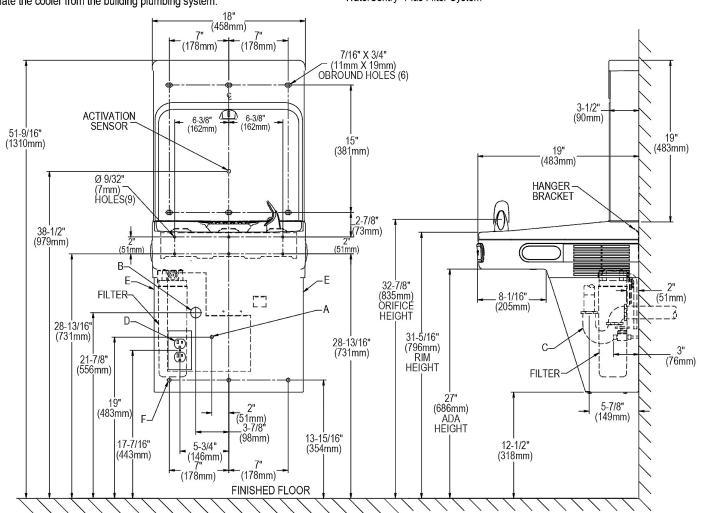
REDUCE HEIGHT BY 3 INCHES FOR INSTALLATION OF CHILDRENS ADA COOLER A = Recommended Water Supply location. Shut-off Valve (not furnished) to accept 3/8" O.D. unplated copper tube. Up to 3" (76mm) maximum out from wall.
