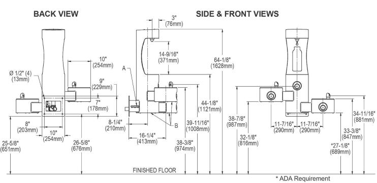
A = 3/8" O.D. UNPLATED COPPER TUBE CONNECT - SHUT OFF VALVE BY OTHERS
