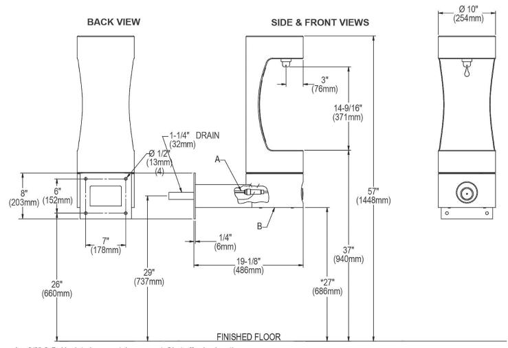
A = 3/8" O.D. Unplated copper tube connect. Shut off valve by others.  $B = Access panel(8" \times 10")$
