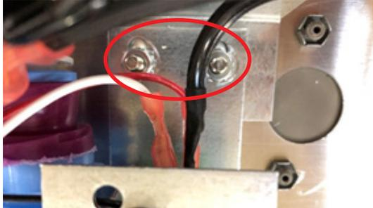
11. Unplug wires from solenoid terminal and remove the solenoid from the aerator connection.
