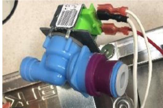
12. Place new solenoid on aerator making sure it is completely seated to prevent leaks. Plug in wires to terminals.
