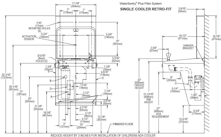
B = Recommended Water Supply location. Shut-off Valve (not furnished) to accept 3/8" O.D. unplated copper tube. Up to 3" (76mm) maximum out from wall. B = Recommended Waste Outlet location. To accommodate 1-1/4" nominal drain. Drain stub 2" (51mm) out from wall.
