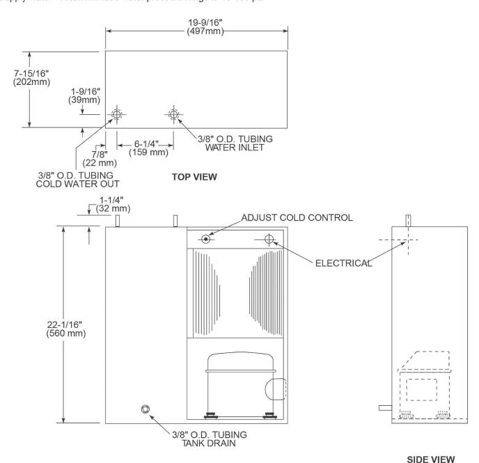
**NOTE**: It is important to insure proper ventilation. Allow a minimum clearance of 6" (152 mm) in front and 3"(76 mm) in the rear of the unit. If unit is to be installed in an enclosure, allow the following clearances around unit: 1"(25 mm) each side, 3"(76 mm) in the rear, 3"(76 mm) above. A 6"(152mm) clearance beyone the front of the wall grill is required.
