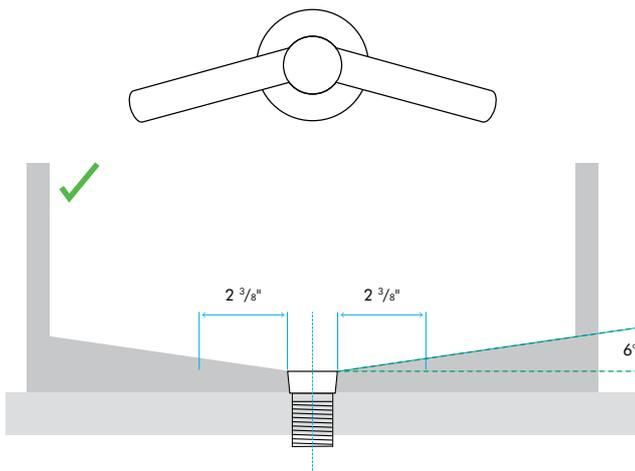
Minimum of  $6^\circ$  ramp angle from the edge of the drain hole of the sink will result in good drainage leading to reduced levels of splashback (minimum  $2\frac{3}{8}$ " radius).
