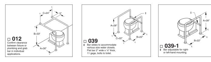
**NOTE:** When Grab Bar dimensions are modified, a support will be added to all sections longer than 54".
