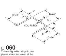
pieces which are joined at the coupling. This configuration can ship via UPS.
