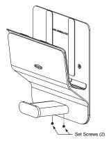
Removing set screws located at the bottom of the hook assembly using Allen wrench (not provided).
