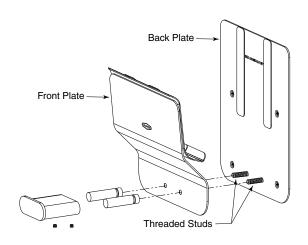
Remove Front-Plate from Back-Plate by pulling the Front-Plate off the threaded studs.
