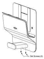
1. Removing set screws located at the bottom of the hook assembly using Allen wrench (not provided).
