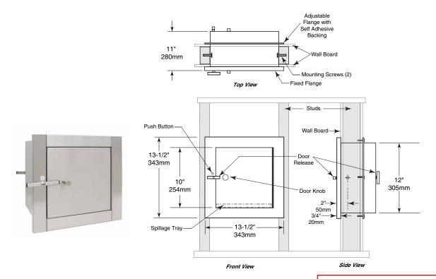
Rough Wall Opening 12-3/8" (315mm) wide 12-3/8" (315mm) high 3" to 10" (76 to 254mm) wall thickness
