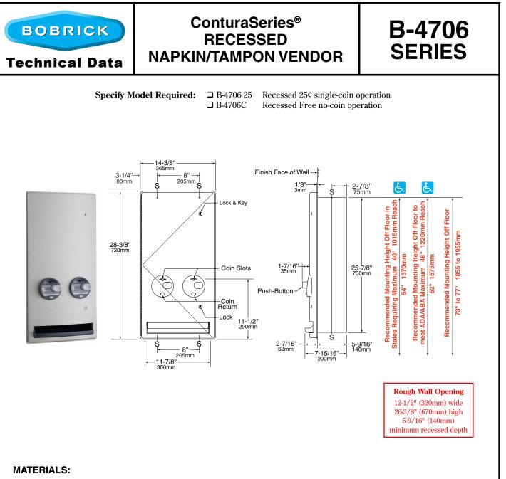
Cabinet — 18-8, Type-304, 18-gauge (1.2mm) stainless steel. All-welded construction.
