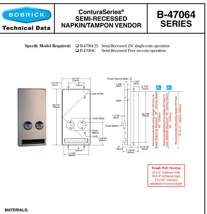
Cabinet — 18-8, Type-304, 18-gauge (1.2mm) stainless steel. All-welded construction.
