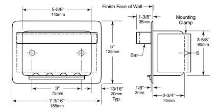
Rough Wall Opening 6" (150mm) wide 4" (100mm) high 4" (100mm) minimum recessed depth
