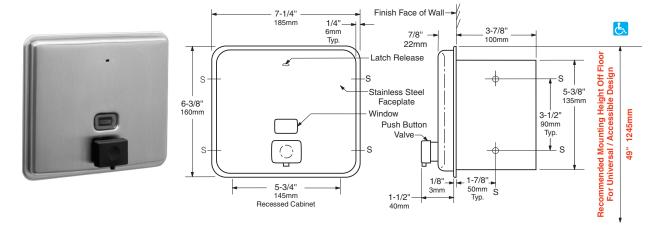
Rough Wall Opening 5-7/8" (150mm) wide 5-1/2" (140mm) high 4" (102mm) minimum recessed depth
