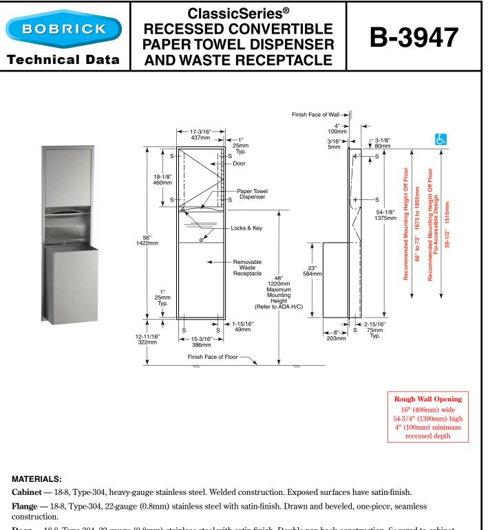
**Door** — 18-8, Type-304, 22-gauge (0.8mm) stainless steel with satin-finish. Double-pan-back construction. Secured to cabinet with a full-length stainless steel piano-hinge. Equipped with a semi-concealed tumbler lock keyed like other Bobrick washroom accessories.
