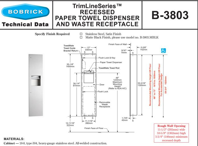
**Door** — 18-8, type-304, 18-gauge (1.2mm) stainless steel.  $9/16^{"}$  (14mm)  $90^{\circ}$  return for maximum rigidity. Secured to cabinet with a concealed, full-length, stainless steel piano-hinge. Equipped with a stainless steel cable door-swing limiter and two tumbler locks keyed like other Bobrick washroom accessories. Tumbler locks flush with the door - no protrusion.
