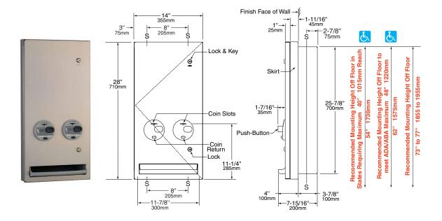
Rough Wall Opening 12-1/2" (320mm) wide 26-3/8" (670mm) high 3-7/8" (100mm) minimum recessed depth
