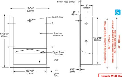
Rough Wall Opening 11-1/4" (285mm) wide 15-5/8" (395mm) high 4" (102mm) minimum recessed depth
