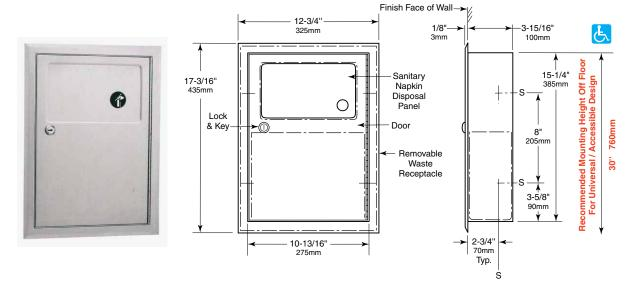
Rough Wall Opening 11-1/4" (285mm) wide 15-5/8" (395mm) high 4" (102mm) minimum recessed depth
