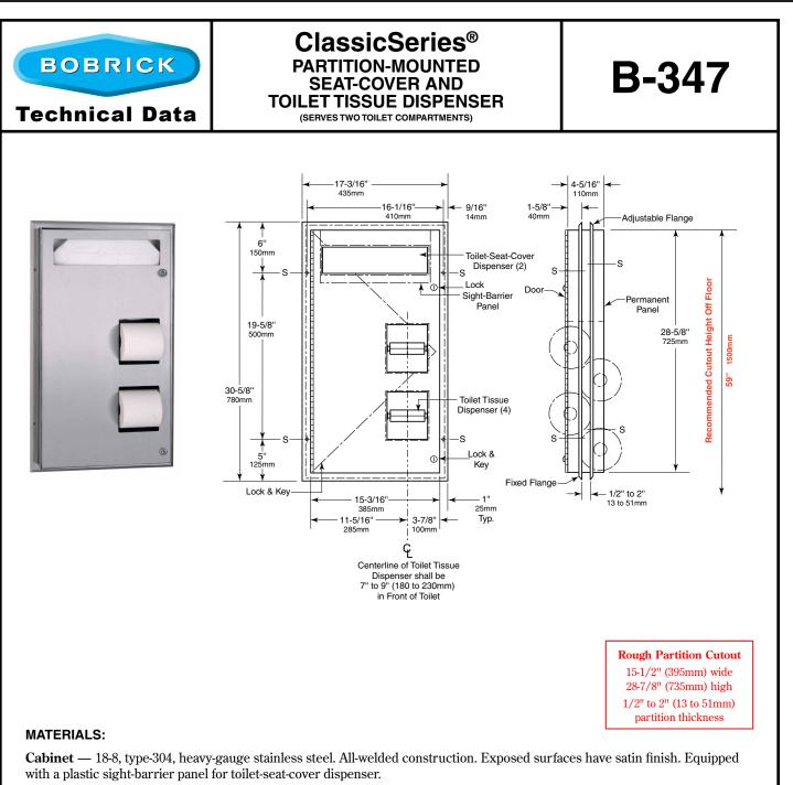
**Flanges (2)** — 18-8, type-304, 22-gauge (0.8mm) stainless steel with satin finish. Drawn and beveled, one-piece, seamless construction.
