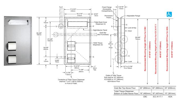
**Note:** For accessible toilet compartments, please use horizontal recessed or surface -mounted combination dispenser-/disposal-units, B-3091 or B-3092 Series, to comply with ADA 1-1/2" absolute Grab Bar wall spacing.
