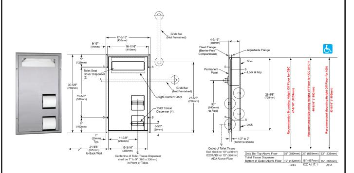
**Note:** For accessible toilet compartments, please use horizontal recessed or surface -mounted combination dispenser-/disposal-units, B-3091 or B-3092 Series, to comply with ADA 1-1/2" absolute Grab Bar wall spacing.
