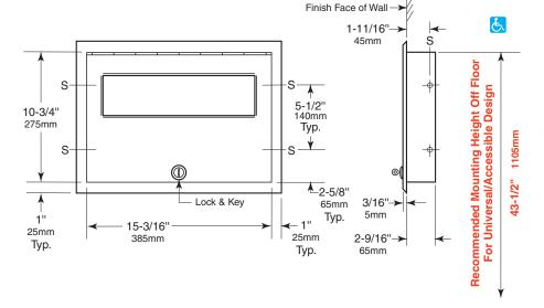
Rough Wall Opening 15-5/8" (395mm) wide 11-1/4" (285mm) high 2-5/8" (67mm) minimum recessed depth
