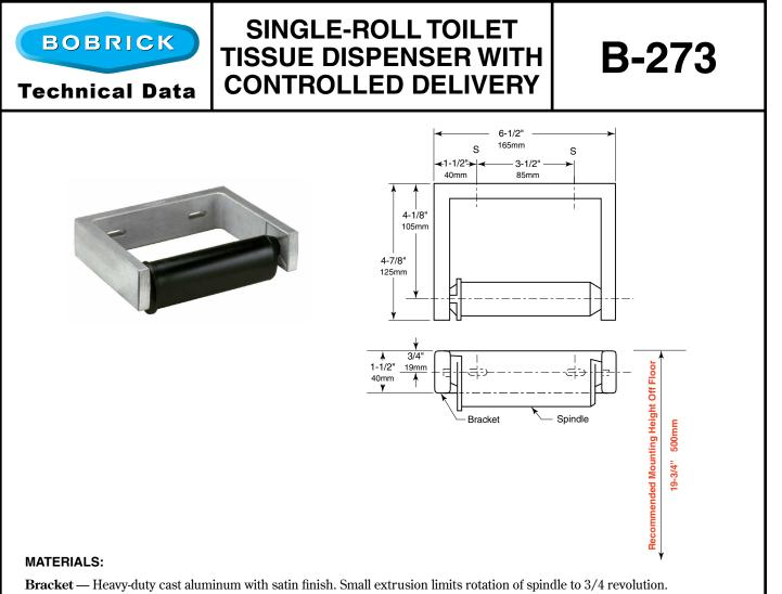
**Spindle** — Molded high-impact ABS. Equipped with retractable pin and concealed locking mechanism.
