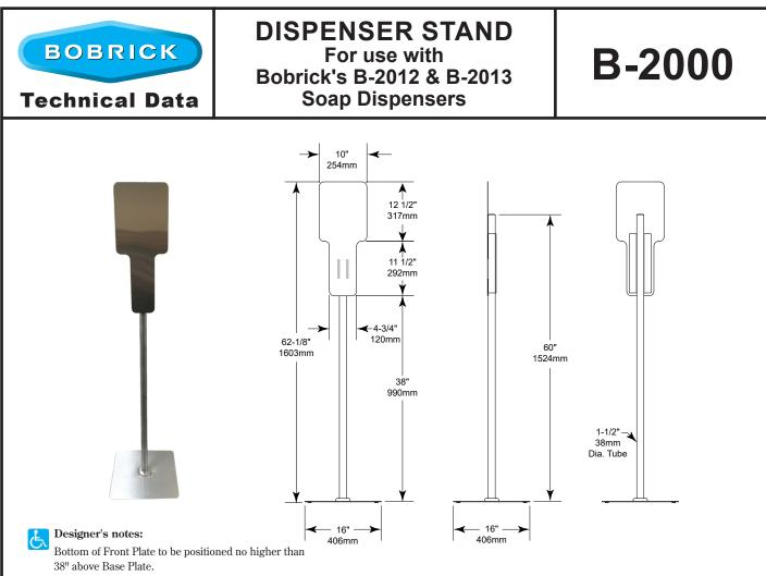
Install dispenser to Front Plate with the bottom of dispenser outlet 40" maximum above floor".
