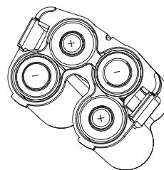
Replace cover of the battery pack assembly and reinsert assembly into faucet.
