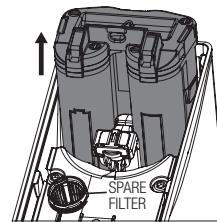
Open battery pack assembly by pushing in tabs on side of assembly.
