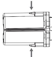
Remove (4) AA-cell batteries from battery pack.
