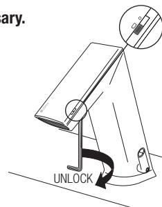
Remove battery pack assembly by lifting out of spout.
