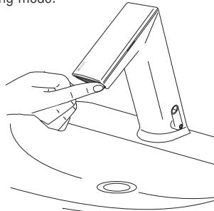
Cover IR clic until LED flashes 4x - hold until LED flashes 1x to 8x, from minimum to maximum. See diagram below. Release when requested range is reached.
