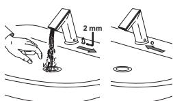
Optional Hot Limit Stop Adjustment — To adjust the hot/cold mix (factory set at 50/50) remove the lever.
