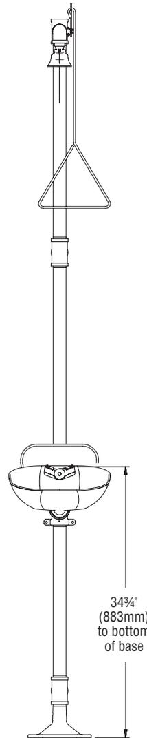
**✓ All dimensions assume standard thread engagement. Variations in manufacturing allow for +/- 1/16" (3mm) per threaded joint. To find the tolerance of a dimension, add the number of thread joints across the length of the dimension and multiply it by 1/16" (3mm).**
