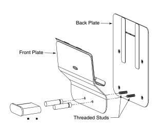
4. Remove Front-Plate from Back-Plate by pulling the Front-Plate off the threaded studs.
