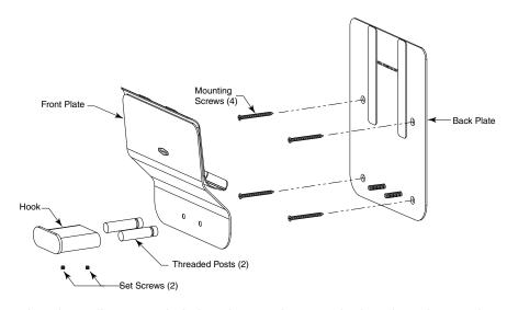
5. Mount unit against the wall at screw hole locations and secure the item by using #8 sheet metal mounting screws (not furnished), length of screw depends on wall-depth (partition-wall to masonry).
