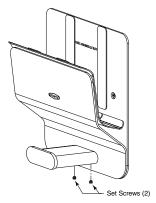
1. Removing set screws located at the bottom of the hook assembly using Allen wrench (not provided).
