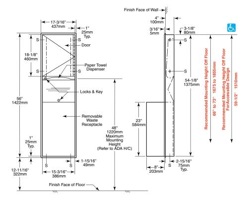
Rough Wall Opening 16" (406mm) wide 54-3/4" (1390mm) high 4" (100mm) minimum recessed depth
