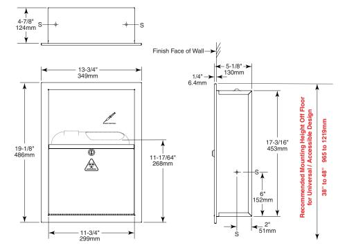
**Rough Wall Opening** 12" (305mm) wide 17-3/8" (441mm) high 5" (127mm) minimum recessed depth
